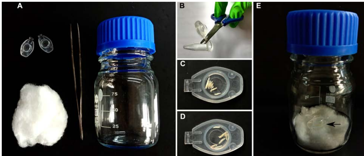
Fig. 1. Setup for immobilizing larvae by ether anesthesia. A. Components of the setup for larval anesthesia. B. Cutting off the cap of 1.5 mL microfuge tube with scissors. C. A few larvae in PBS in the space in microfuge tube cap. D. Larvae in the cap after aspirating out of the PBS. E. Larvae in the cap (arrow) being exposed to ether in the closed bottle with ether-soaked cotton.
